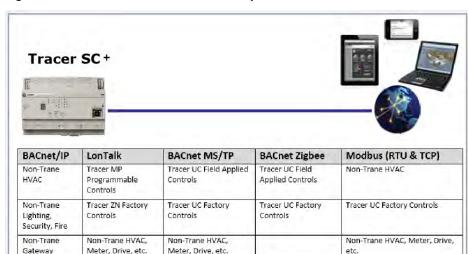
Figure 1. Tracer BAS structure (PC/tablet/phone with web browser)
